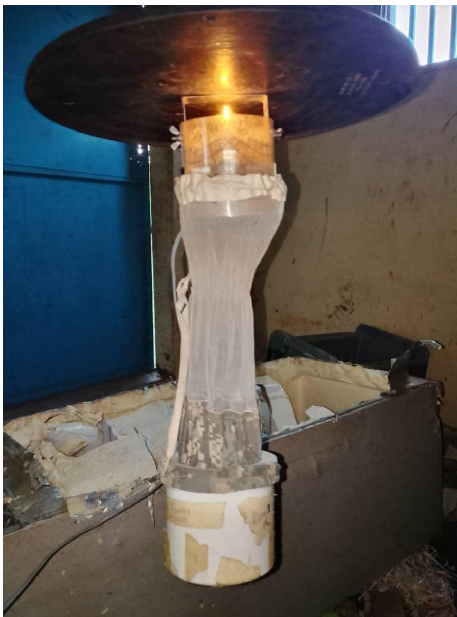
CDC light trap set up for adult mosquito collection at sentinel households as part of routine surveillance.
