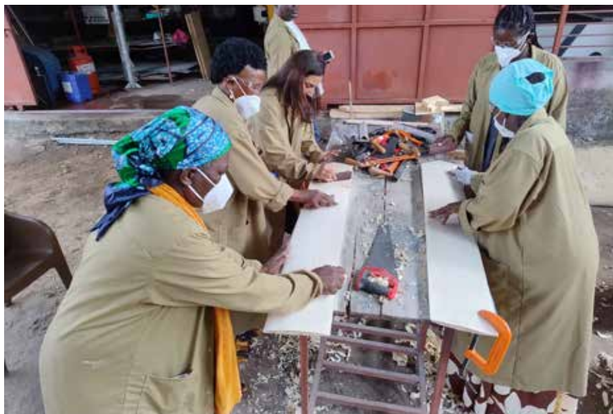
Women cutting blades (Workshop photo). Women artisans in Dar es Salaam hand-carve turbine blades during our Energy in a Box workshop, gaining practical skills in locally manufacturing clean-energy technology.
