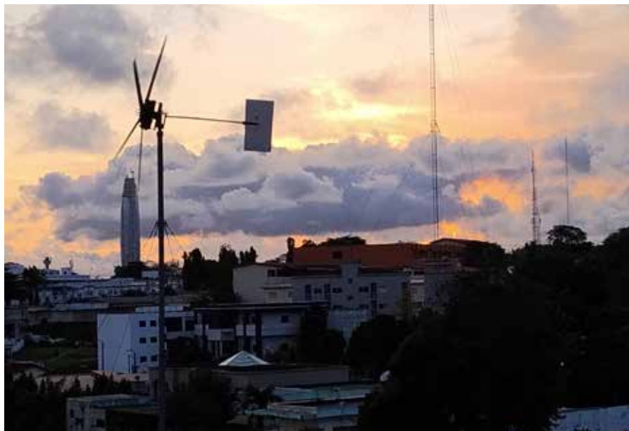
Framed by the Abidjan skyline, this 500-watt wind turbine undergoes performance testing – an essential step before any unit is deployed to the field. This model was tested in preparation for our workshop in Tanzania.
